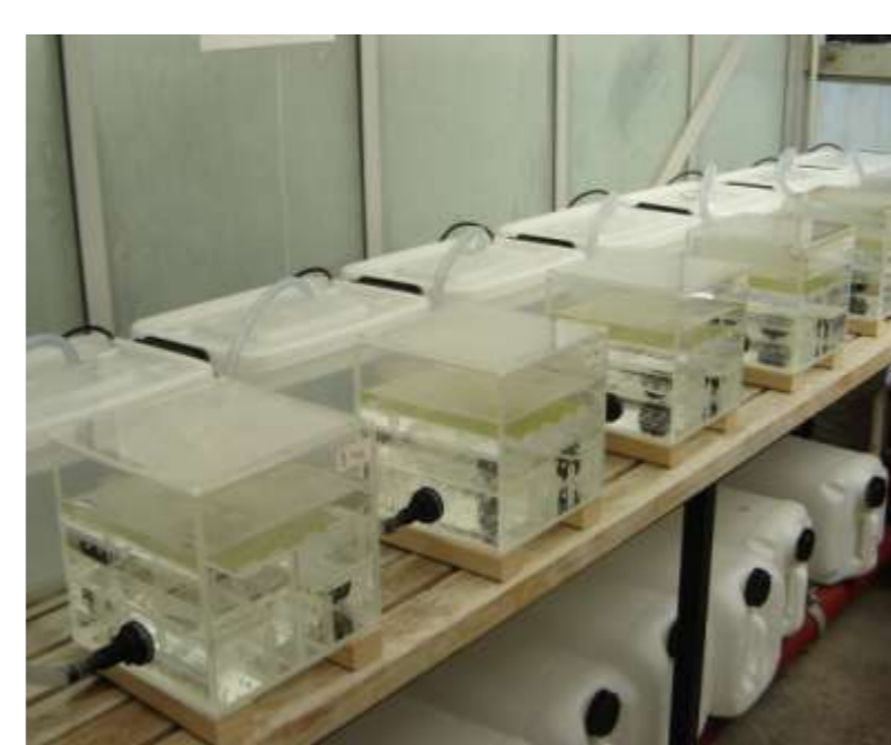
Flow chamber microcosms: a water pump makes the water flow above the biofilm to simulate a natural stream flow.
